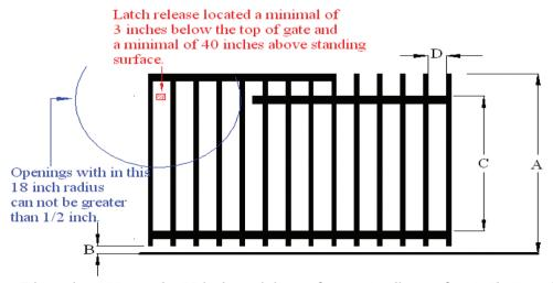
Dimension "A" must be 48 inches minimum from a standing surface to the top of gate. Dimension "B" may be 2 inches maximum from standing surface to the bottom of gate. If dimension "C" is less than 45 inches, dimension "D" cannot be greater than 1-3/4 inches. Dimension "D" can never be greater than 4 inches.
