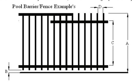
Dimension "A" must be 48 inches minimum from a standing surface to the top of fence. Dimension "B" may be 2 inches maximum from standing surface to the bottom of fence. If dimension "C" is less than 45 inches, dimension "D" cannot be greater than 1-3/4 inches. Dimension "D" can never be greater than 4 inches.
