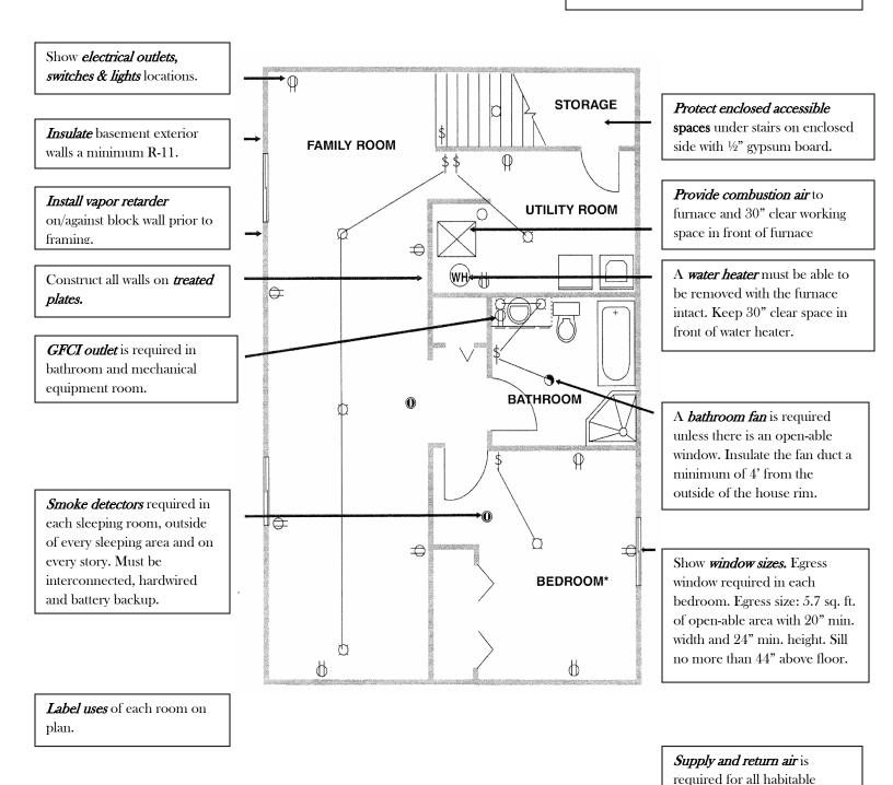
Minimum *ceiling height* is 7' with 6'-8" allowed for projections such as beams and ducts.
