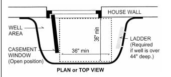
**Note:** Centering a window well at the window might not give you the *required* minimum 36 inches. **Measure carefully!**
